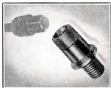
The "Belling-Lee" suppressor L630 screws into specified makes of distributor caps after removal of the H.T. lead terminal, which is then screwed into the top of the suppressor.
